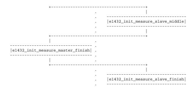
Why is this so complex? Why use separate processes? Normally you wouldn't. But some applications might want to deal with separate channel groups using separate processes, and still provide for all of the modules in all of the groups running synchronously. This is what is needed to deal with that.
